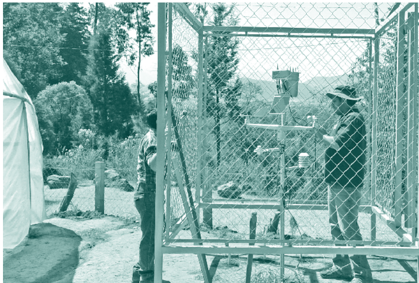
This weather station monitors precipitation, temperature and wind to relay weather information to farmers.
